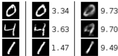
Figure 3. Examples of reconstructed digits from the MNIST dataset with an RBM trained on 60,000 examples for 1 epoch. Left: Original image. Middle: Reconstruction with a 300 hidden units RBM. Right: Reconstruction with a 10 hidden units RBM.
